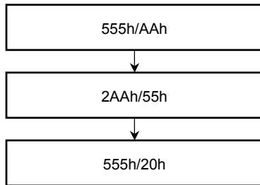
Fast Program Set Command Sequence (address/data)
